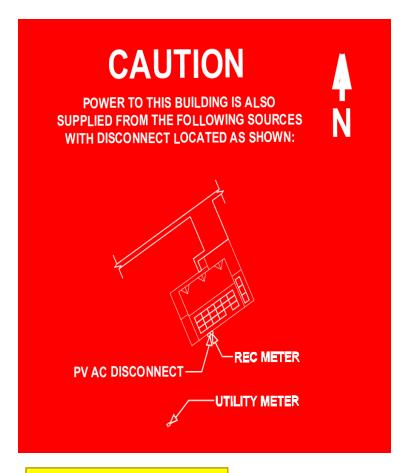
on Billing Meter and on Production Meter, only when billing meter is not attached to the house. (If no Production Meter, place on AC Disconnect), showing any fences.
