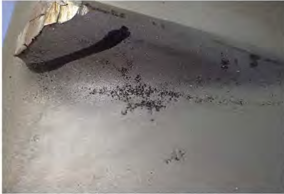
Figure 1. Showing a line of concentrated pitting parallel to the snubber.
