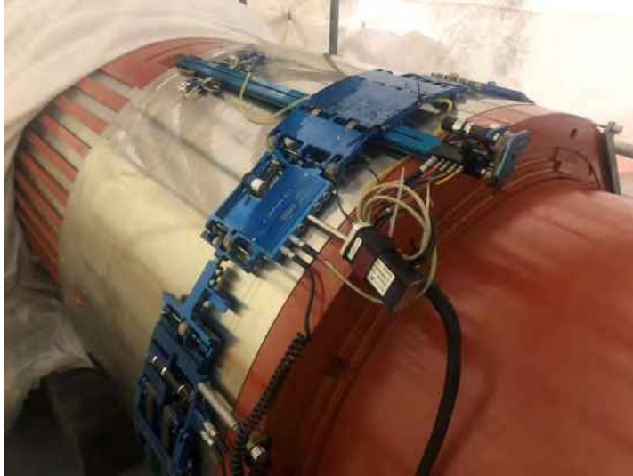
The KIRR 3 manipulator mounted on the turbine side retaining ring.
